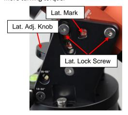
Two latitude ranges, 14~44° and 36~68°, can be set up for the mount head. To change the latitude range
