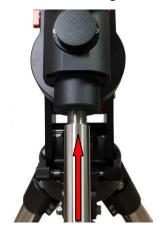
5. Install Counterweight(s): Before putting on CW, make sure the mount is at its zero position, i.e., CW shaft points to the ground. Disengage the R.A. Gear Switch to set the R.A. axis free before loading the CW. Remove the CW Safety Cap at the end of CW Shaft. Glide the CW over the shaft. Tighten the CW Locking Screw to hold the CW in place. Place the Safety Cap back onto the shaft. Move the CW to the bottom of the shaft and tighten the CW locking Screw.
